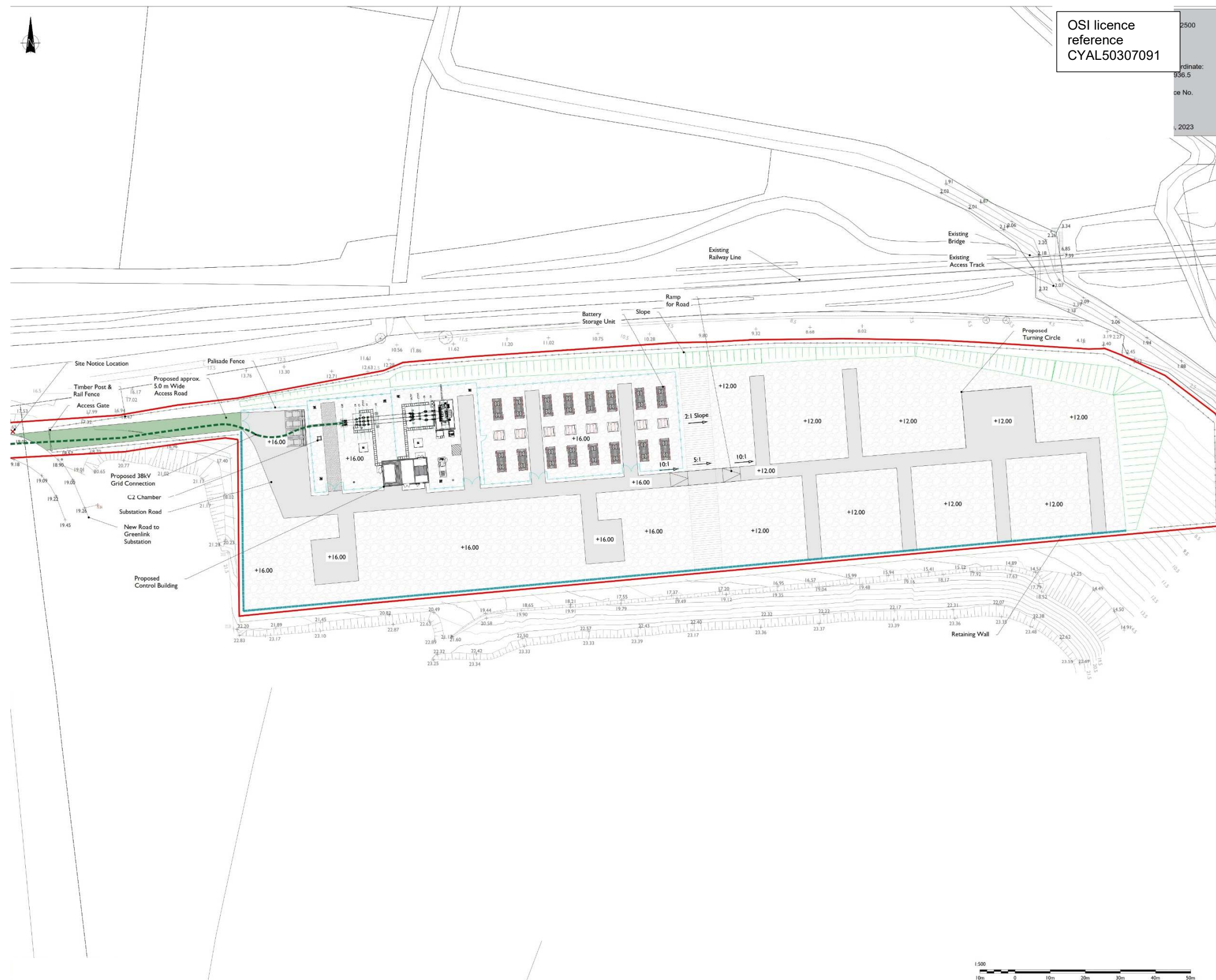
Figure A1 Proposed 30 MW BESS and 38kV Substation Site Layout Plan (From TLI Group Drawing Ref. 09551-DR-302 Rev. P2 29.09.2023)
